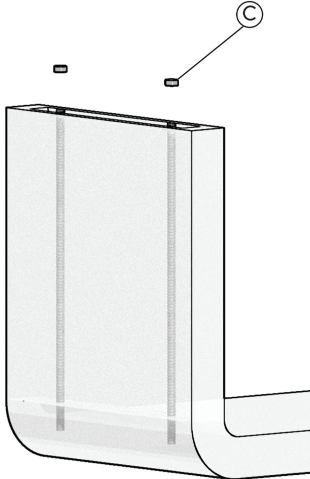
Fix the screw and gasket,
