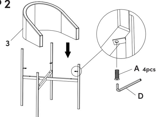
Install the rear two screws first; then the front two screws next.
